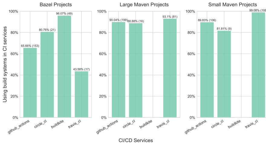
Fig. 11 The percentage of projects in the dataset adopting a CI service and using the Maven or Bazel build system in CI. A project may be counted multiple times if it uses multiple CI services.
